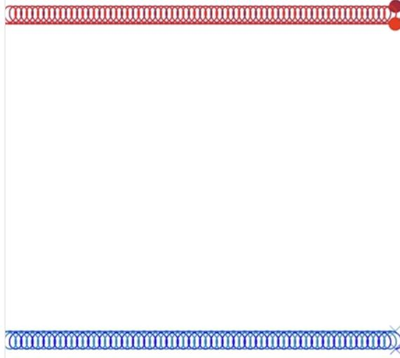
FIGURE 5.1. Vortex pair with double vorticity.
